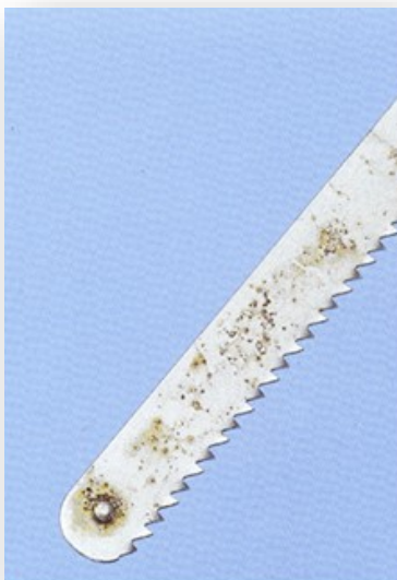
Figure 15: Discolouration and Rusting due to poor cleaning
