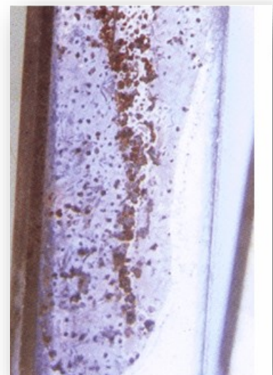
Figure 17: Pitting due to Caustic Solution—magnified
