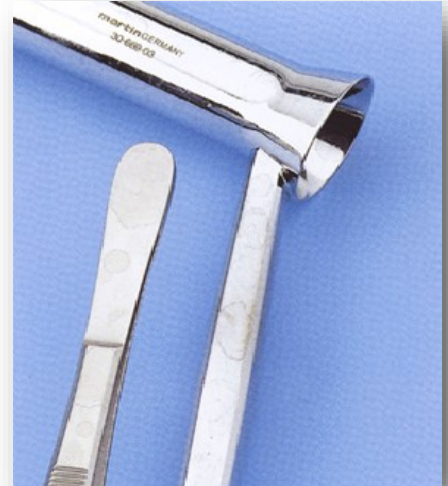
Figure 8: Staining due to a high Concentration of minerals.
