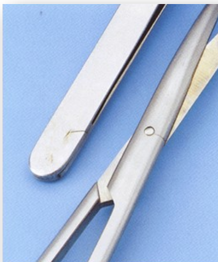
Figure 10: Stress Corrosion Cracking
