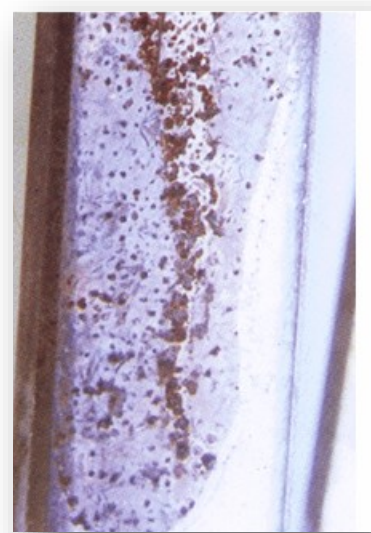
Figure 17: Pitting due to Caustic Solution—magnified
