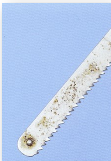
Figure 15: Discolouration and Rusting due to poor cleaning
